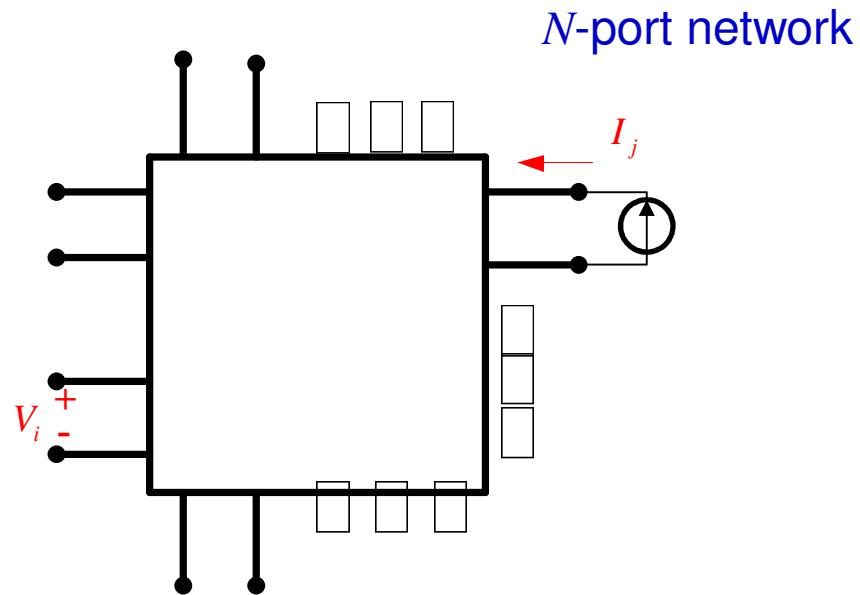
We inject a current into port  $j$  and measure the voltage (with an ideal voltmeter) at port  $i$ . All ports are open-circuited except  $j$ .
