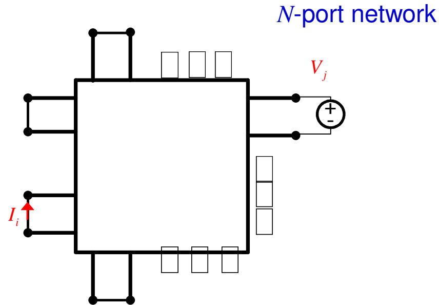
We apply a voltage across port *j* and measure the current (with an ideal current meter) at port *i*. All ports are short-circuited except *j*.
