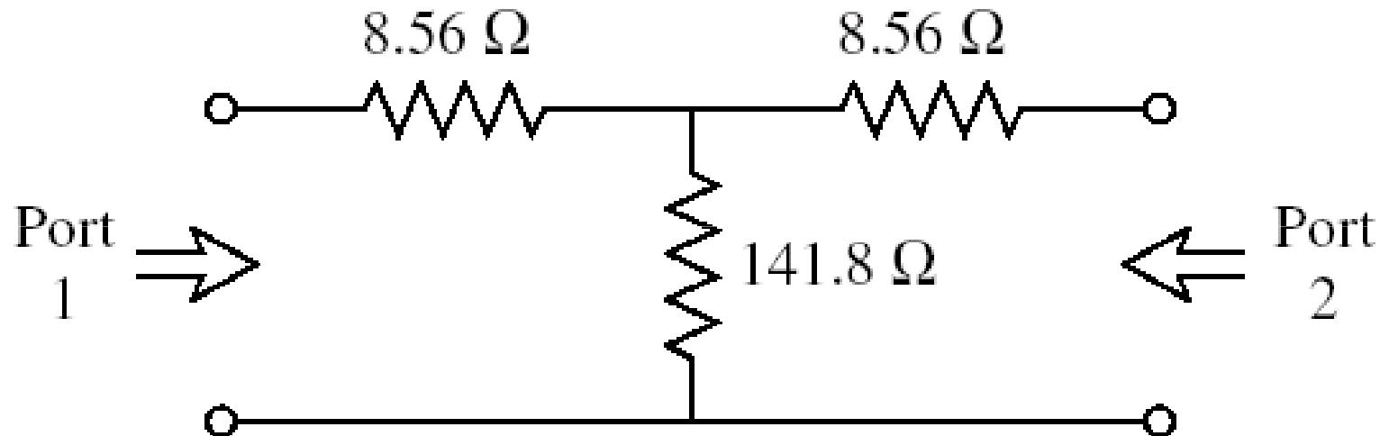
A matched 3B attenuator with a  $50 \Omega$  Characteristic impedance
