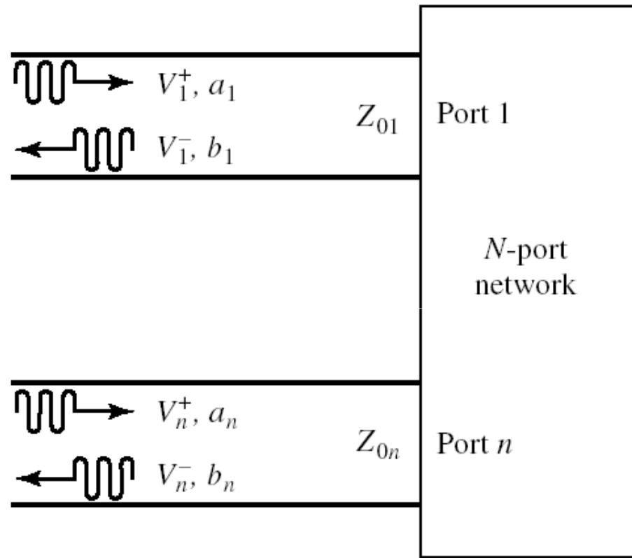
An  $N$ -port network with different characteristic impedances.
