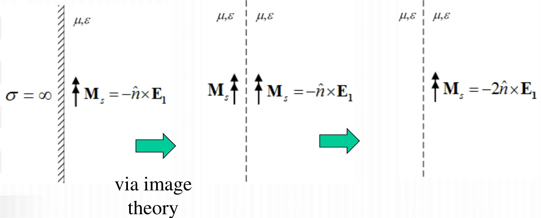
Equivalent models for magnetic source radiation near
