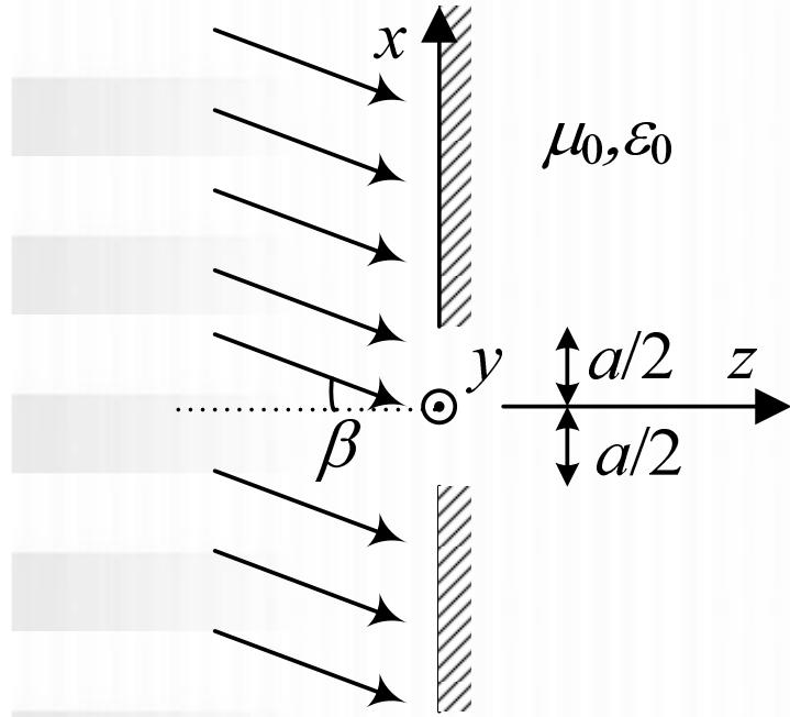
A uniform plane wave traveling in the direction as shown. The field is given by
